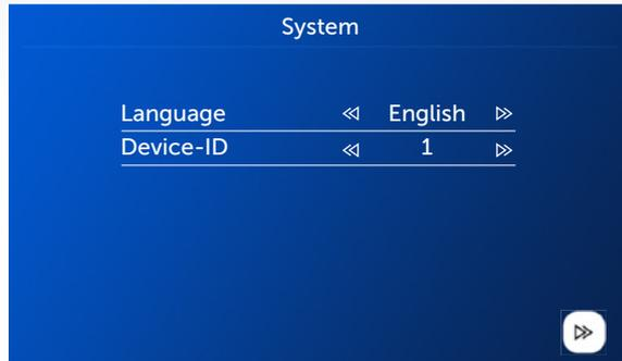
**Please note:** The Device ID is an important configuration of the equipment in the system. It must be configured correctly, otherwise it will not work properly. If the current device is connected to the Outdoor unit 1, it must be set to 1, and the others Slave monitors must be set 2/3/4/5/6 to work normally.
